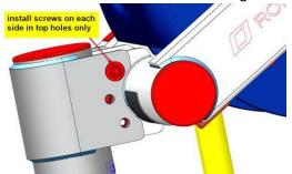
3. Following illustration in #2 above please install 2 screws as shown (one on each side) and use the head as a lever to tilt and align holes
