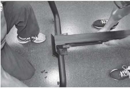
**6.** Attach the front curved tubular floor brace to the post. Using four hex head bolts  $3/8'' \times 5/8''$  long bolts, screw down until firmly tight.
