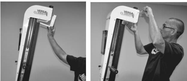
**19.** With the post supported or after VersaClimber is upright, slip pump cover into place. Attach with four Phillips pan head screws 1/4" x 1/4" long. **DO NOT OVER TIGHTEN.**
