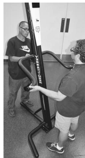
**17.** Attach side handrails with (3) hex head bolts 4" long and (3) 3/8" lock nuts.
