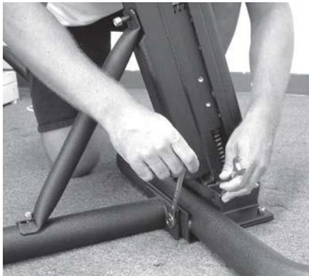
**12.** After tubular brace is in place, go back and **FULLY TIGHTEN** the (2) 3 ¾" long base bolts.
