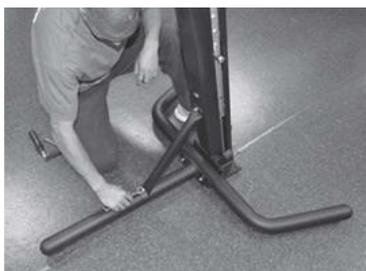
**14.** Next, tighten the **BOTTOM** lock nut on the back brace to complete post assembly.
