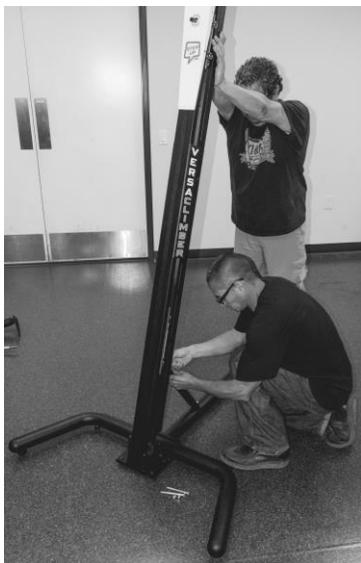
**13.** Then go back and **TIGHTEN FULLY** the TOP lock nut on the tubular brace.
