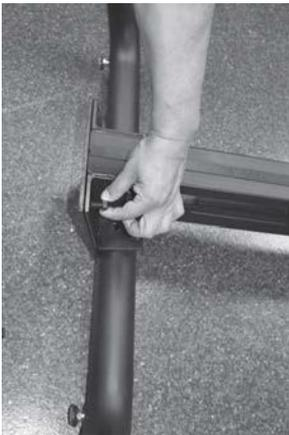
**7.** Screw in (4) self tightening base bolts.
