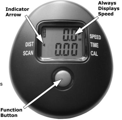
The *Indicator Arrow* points to the function that is being displayed. For example, in the picture the *Indicator Arrow* is pointing to DIST, so the lower number displays the total distance rope has been pulled.
